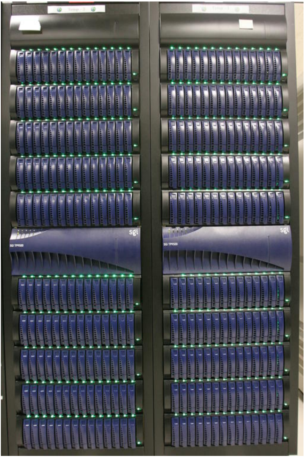
Columbia's storage is 440TB of disk, some Fibre Channel, some Serial ATA. The system already has 650 users at Ames and at cooperating universities and national labs.
